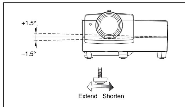
**14 LENS SHIFT knob / SHIFT LOCK fixing bolt**
